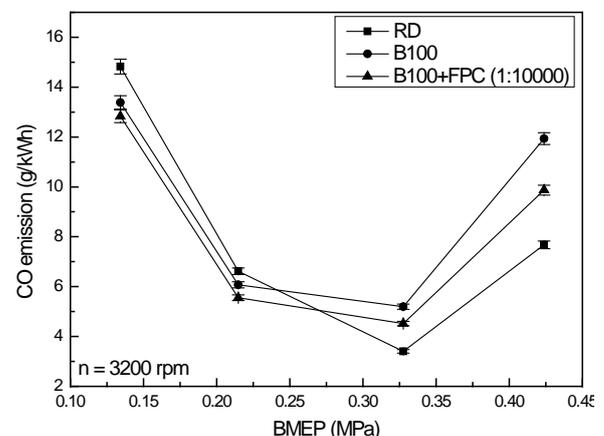
Figure 3 Variation of CO emissions as a function of engine load for the three fuels at the speed of 3200rpm
