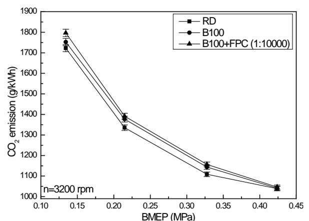
**Figure 5** Variation of CO<sub>2</sub> emissions as a function of engine load for the three fuels at the speed of 3200rpm
