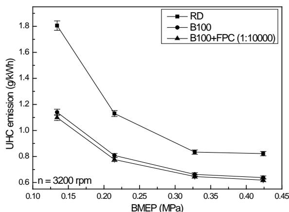
**Figure 4** Variation of UHC emissions as a function of engine load for the three fuels at the speed of 3200rpm
