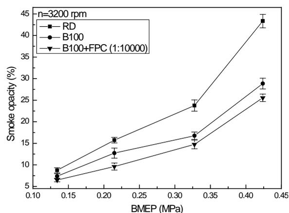
**Figure 2** Variation of smoke emissions as a function of engine load for the three fuels at the speed of 3200rpm
