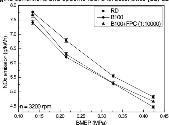
**Figure 6 Variation of NO<sub>x</sub> emissions as a function of engine load for the three fuels at the speed of 3200rpm**
