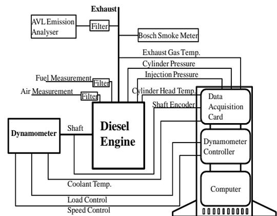
Figure 1 Schematic diagram of the engine test system
