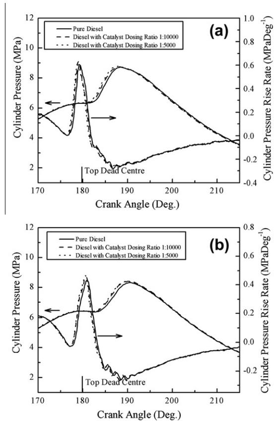
Fig. 6. In-cylinder pressure and pressure rise rate of the engine with the pure diesel and diesel dosed with the catalyst. (a): engine speed: 2800 rpm and engine load: 0.4 MPa; and (b): engine speed: 3200 rpm and engine load: 0.42 MPa.
