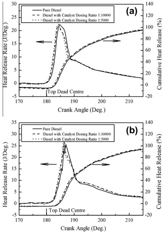
**Fig. 7.** Heat release rate and cumulative heat release of pure diesel and the diesel dosed with the catalyst. (a): engine speed: 2800 rpm and engine load: 0.4 MPa; and (b): engine speed: 3200 rpm and engine load: 0.42 MPa.
