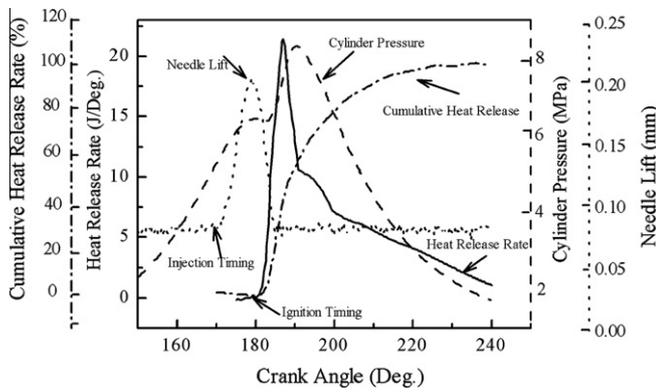
Fig. 2. Definitions of combustion characteristics in diesel engines.
