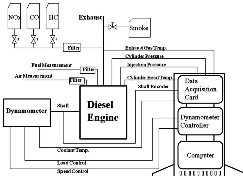
Fig. 1. A schematic diagram of the diesel engine test bench.
