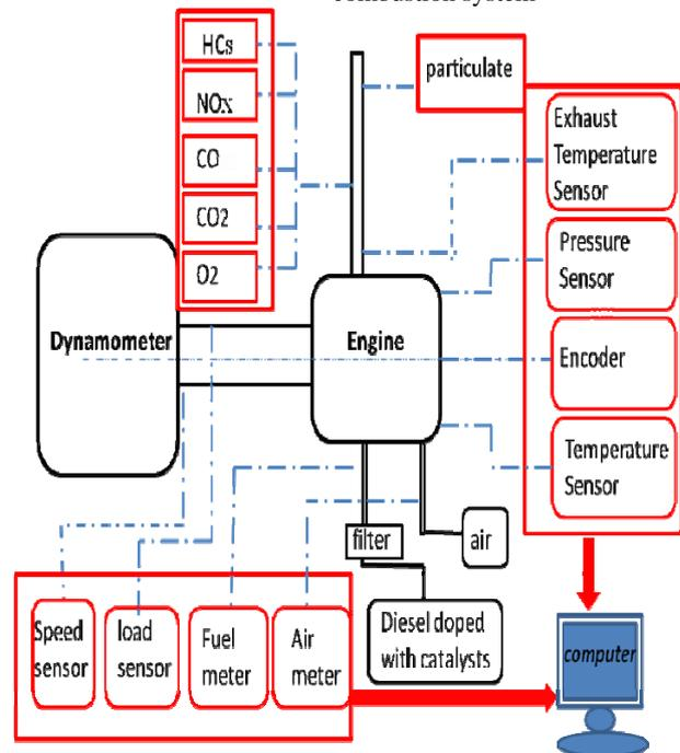
Figure 3 A flow sheet diagram of laboratory controlled engine test system
