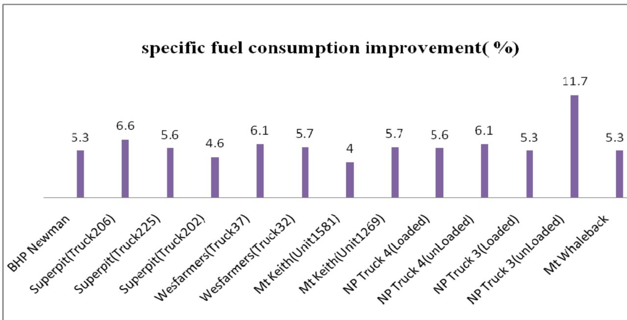
Figure 1 Effect of homogeneous combustion catalysts on specific fuel consumption improvement in diesel engines(NP: Norwich Park mine)
