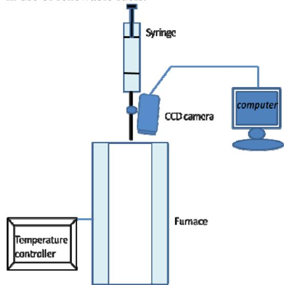
Figure 2 A schematic diagram of diesel droplet combustion system
