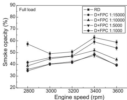
Fig. 2. Variation of the smoke emissions as a function of engine speed for the five fuels tested under the full load conditions.
