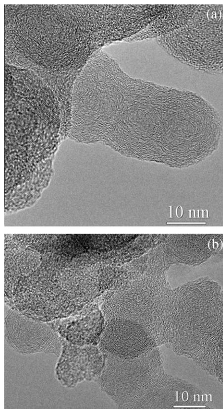
Fig. 7. High-resolution TEM images (250,000 $\times$ ) of soot particles from (a) reference diesel and (b) diesel with FPC at 1: 10<sup>4</sup> dosing ratio.
