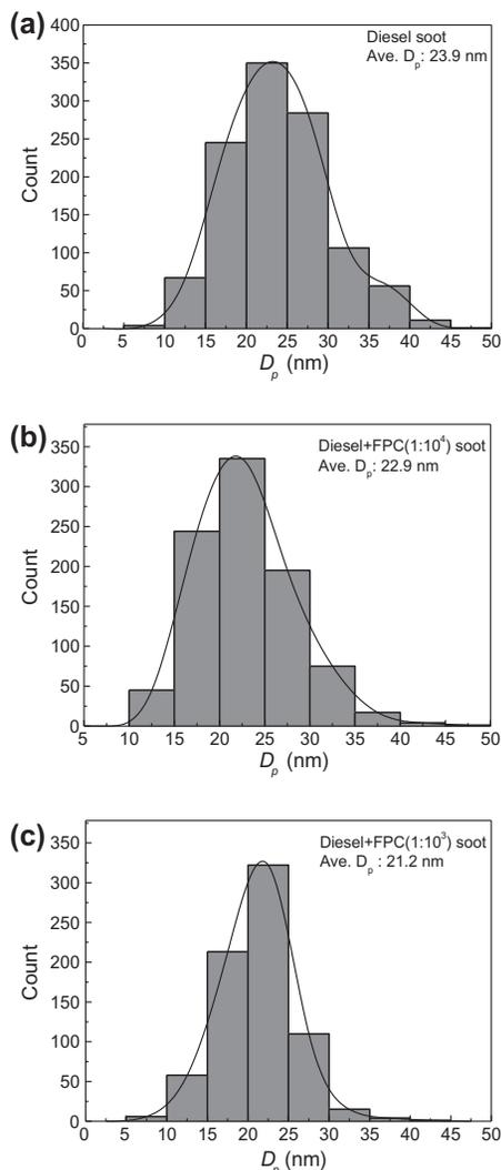
Fig. 6. The primary particle size distributions of soot samples from (a) reference diesel, (b) diesel with FPC at 1: 10<sup>4</sup> dosing ratio and (c) diesel with FPC 1:10<sup>3</sup> dosing ratio under the engine speed of 3200 rpm and 5.5 Nm load condition.
