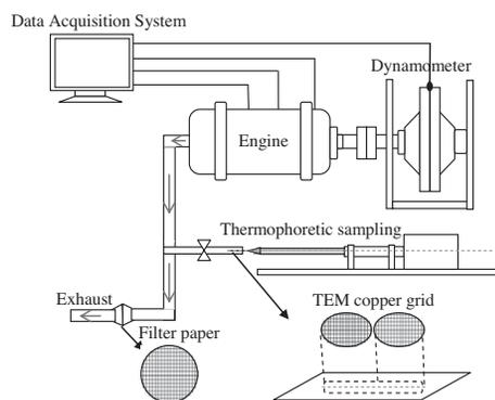
Fig. 1. A schematic of the arrangements for soot sampling and collection.
