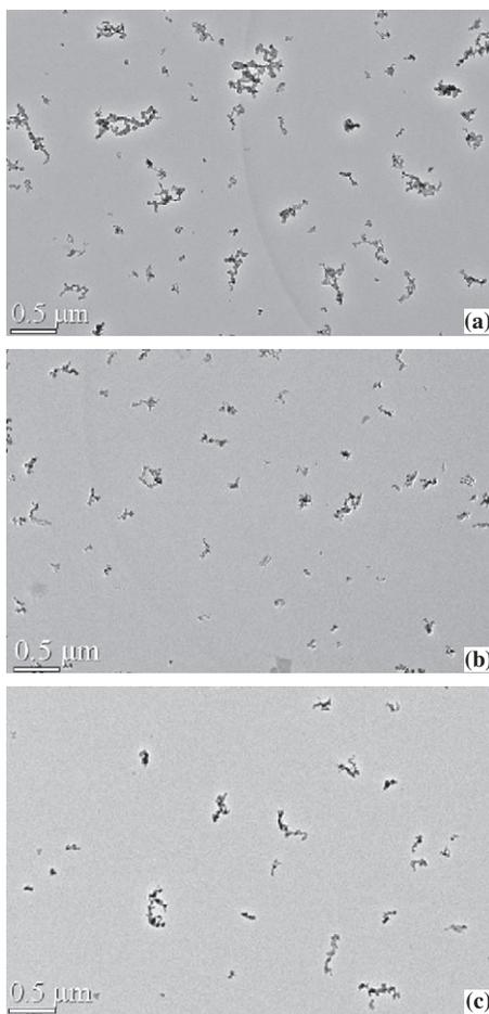
Fig. 5. Low magnification TEM images (5000 $\times$ ) of soot samples from (a) reference diesel, (b) diesel with FPC at 1:10<sup>4</sup> dosing ratio and (c) diesel with FPC 1:10<sup>3</sup> dosing ratio under the engine speed of 3200 rpm and 5.5 Nm load condition.
