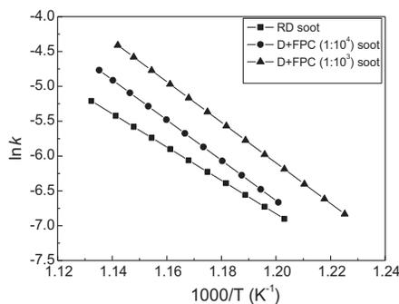
Fig. 4. Arrhenius plots for the oxidation of the soot samples from diesel with or without the FPC catalyst.
