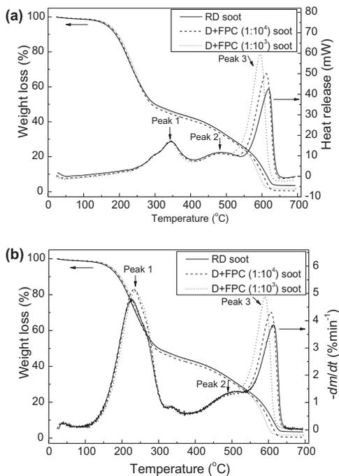
Fig. 3. Comparison of the (a) TG-DSC and (b) TG-DTG curves of the soot samples from the engine operating at 3200 rpm and 5.5 Nm load, and fuelled with diesel with or without FPC catalyst in air.
